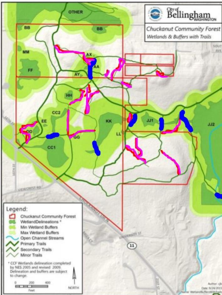
Figure 3 (left): Map of trails to be closed and where wetland mitigation structures are to be installed. Closed trails are marked in pink. Assume any newer trails not on this map are to be closed as well. Wetland mitigation structures are marked in blue. In areas where the trail crosses a wetland or visible connection between wetlands, boardwalks are to be installed and the soil in those areas decompacted. Original map from Eissinger
